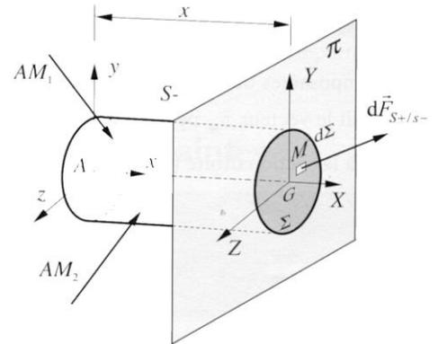
$$\vec{C}_{(M, \vec{x})} = \frac{d\vec{F}}{d\Sigma} = \vec{\sigma}_M + \vec{\tau}_M \quad \text{tel que} \quad \begin{cases} \sigma : \text{contrainte normale} \\ \tau_M : \text{contrainte tangentielle} \end{cases}$$
